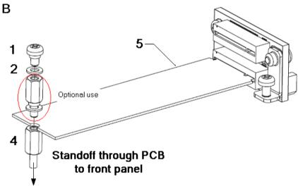
4. Insert the washer (2) and screw (1) into the standoff using the Phillips head screwdriver and torque to 0.1 N-m.
