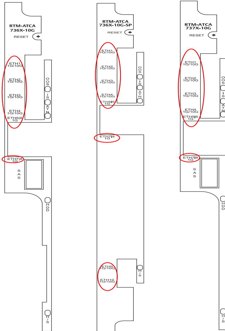
Figure 3-5 Location of Ethernet Connector
